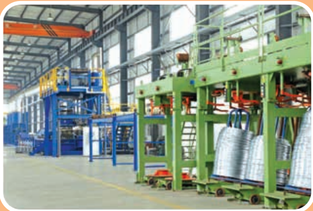
Galvanized Steel Wire Production Line in Heshan, Guangdong, Chinese Mainland
